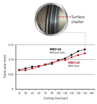
Vibration occurred when using an insert without hole after 165 sec due to high cutting loads.
