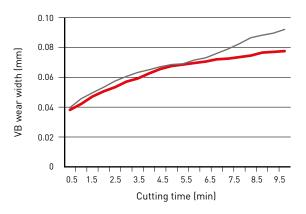
Gives both outstanding wear and fracture resistance, thereby enabling MBS140 to achieve a long tool life without abnormal fracturing even at large depths of cut.
